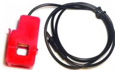
Figure 5. Power Consumption Sensor.
